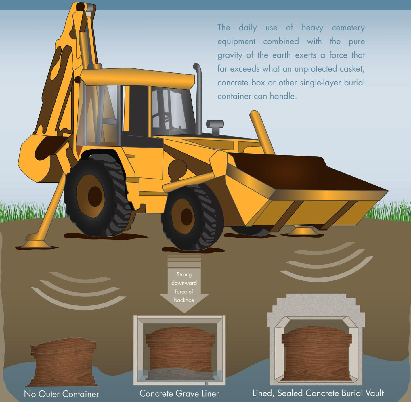
A backhoe can weigh up to 14,000 pounds. An impact load is produced by the dropping of a backhoe bucket and exerts an even stronger force throughout the soil.
